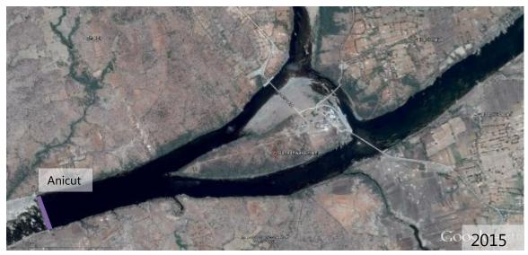
The erosion On Edge1 and Edge 2 is due to the combined discharge of Mahi,Som and Jhakham that passes through the anicut as there is no slope stabilization on the edges making the island shrink in size. Major dams i.e Mahi Bajar Sagar Dam(Peak flood discharge 8.22 lakh cusecs) Som Kamla Amba Dam Dam(Peak flood discharge 7.24 lakh cusecs) Jhakam Dam(Peak flood discharge 4.22 lakh cusecs) are in upstream of anicut.
