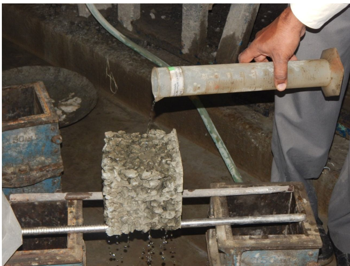
Image 54 No fines concrete experiment in the laboratory (Source- Structwel Laboratory, Mumbai)
